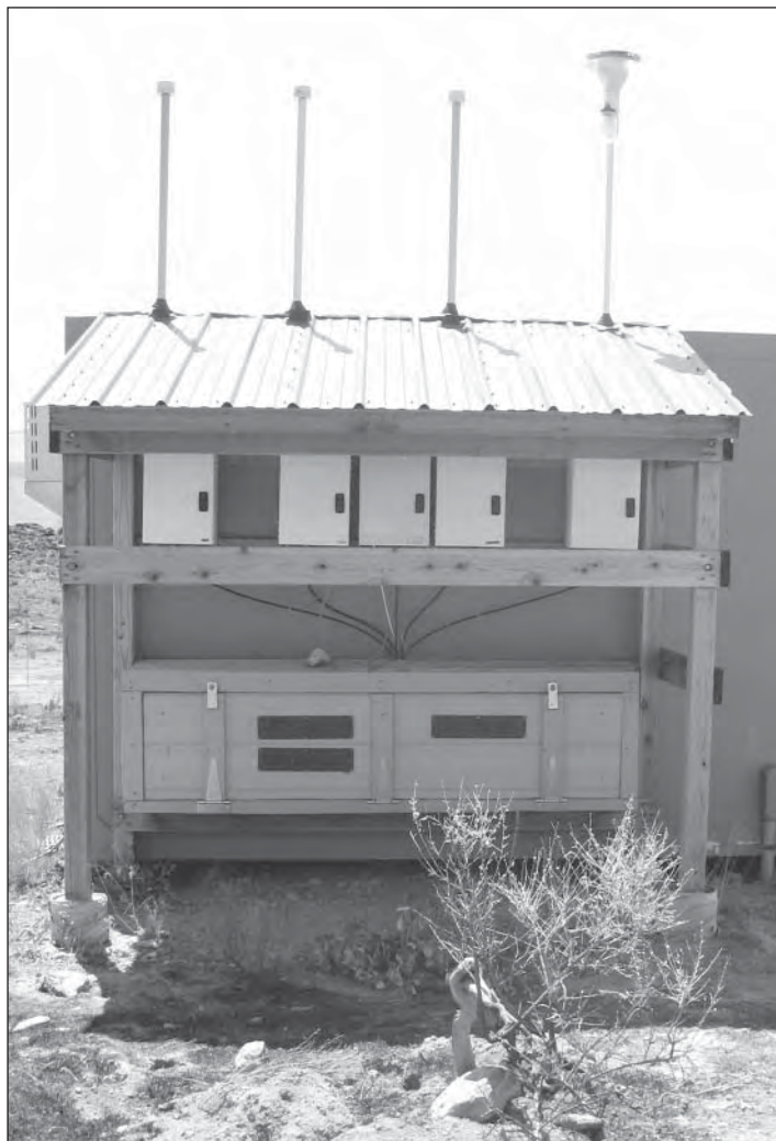
Figure 1. The four-module IMPROVE Version II aerosol sampler installed underneath a lean-to type structure at Zion National Park, Utah.
